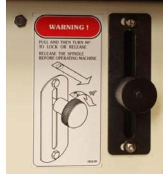
We supply a ½” and ¾”-diameter spindle with the JET JWS-25X shaper (left). Each spindle comes with a full set of spacers. Changing spindles and cutters is made easier because of this external spindle lock (right) on the right side of the cabinet.
