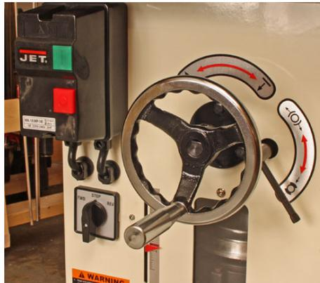
The motor is controlled by a pair of switches on the front of the base cabinet. Because the JET JWS-25X Shaper motor is reversible, we added a three position switch that allows selecting forward, off or reverse.
