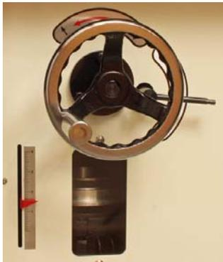
The handwheel and scale allow making precise cutter height changes quickly.
