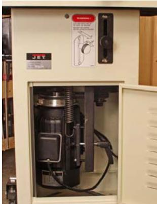
The powerful 3HP motor (left) and its mount are easily accessible through the side door. The major controls are on the front of the cabinet (right), including the magnetic switch that protect the motor and you.
