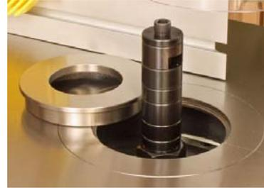
Two high-precision insert rings allow you to size the table opening to fit the cutter.
