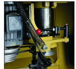
*Five spindle speeds (3,000 to 10,000 rpm) with speed indicator. Fast speed change and tensioning device and big 7½HP motor.*
