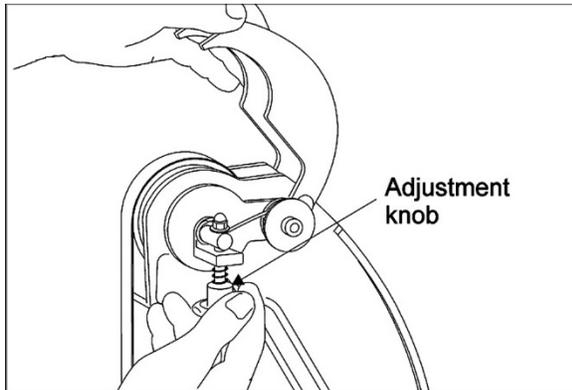
Figure 10: Adjusting belt tracking
