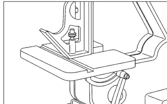
Figure 12: Setting belt table to 90-degree angle
