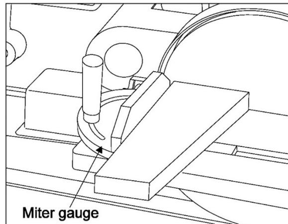
Figure 23: Miter gauge (shown on disc table)
