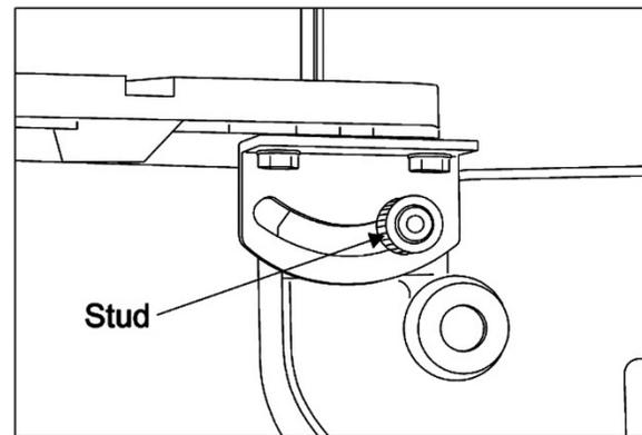
Figure 2: Installing stud in table bracket
